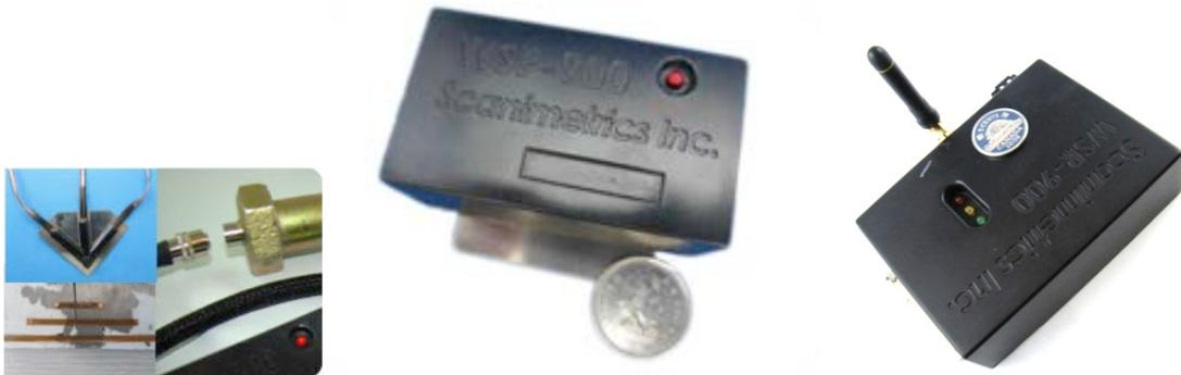
Figures 4a, 4b and 4c: Scanimetrix sensors, wireless sensor modules (Motes) and master Gateway.
